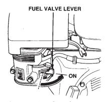
Figure 10. Fuel Shut-OFF Lever
